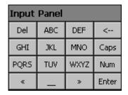
The **«Caps»**, **«Num»** and **«Sym»** buttons can be used to toggle between the different characters (normal characters, numbers and special characters). Each button is assigned with several characters. You operate the buttons in the same way as on a mobile phone – touch once to transfer the first character, twice to transfer the second etc.
